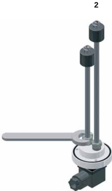
Secure the level indicators to the connector support by means of the ferrule system (14 mm wrench).
